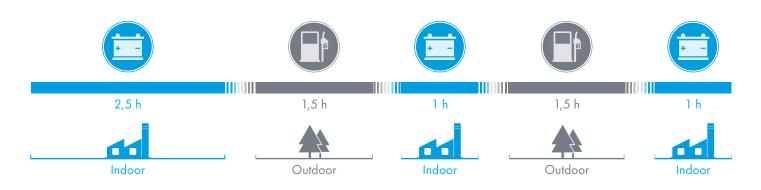
THE HYBRID TECHNOLOGY ENABLES THE OPERATOR TO SWITCH FROM ONE POWER SUPPLY TO THE OTHER, GUARANTEEING UP TO 7.5 HOURS OF CONTINUOUS WORK. THE BATTERIES ARE CHARGED AUTOMATICALLY WHEN THE GASOLINE MOTOR IS USED.
