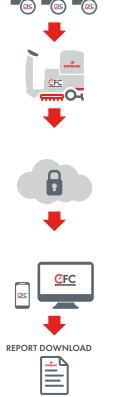
You can choose to assign a tag to each user or a tag to each individual machine. Once the tag has been inserted, the machine can start working as it acts as an additional key.
